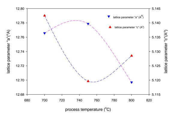
Figure 2 The variation of lattice parameters " a " and " c " with process temperature of the  $Pb_2MnO_4$  ceramics
