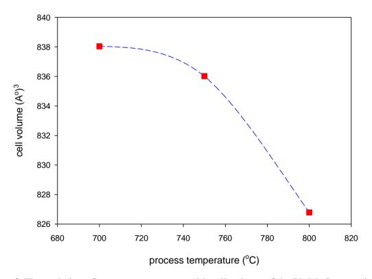
Figure 4 The variation of process temperature with cell volume of the Pb<sub>2</sub>MnO<sub>4</sub> ceramics
