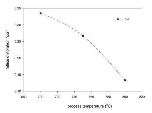
Figure 3 The variation of process temperature with lattice distortion (c/a) of the  $Pb_2MnO_4$  ceramics
