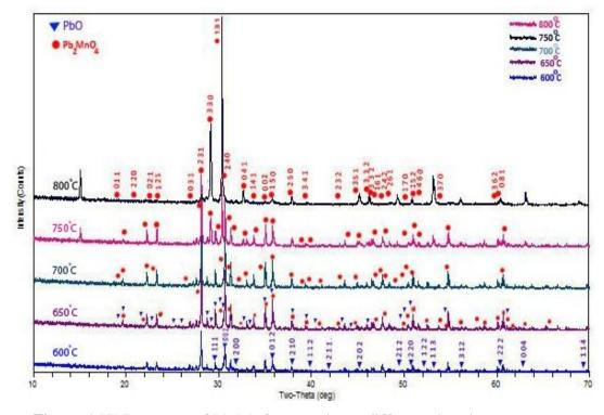
Figure 1 XRD spectra of Pb<sub>2</sub>MnO<sub>4</sub> ceramics at different sintering temperatures.
